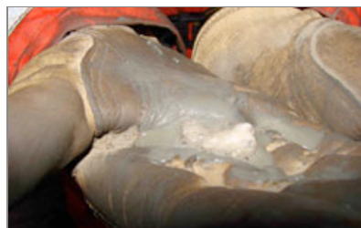
A sample of methane hydrate from a core of the sub-seabed sediment, taken from the methane plumes, where the higher pressure in deeper water keeps the hydrate stable.
